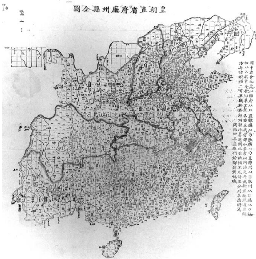
Maps and Mapmaking in China. Fig. 4 Huangchao zhi sheng fu ting zhou xian quantu (Complete Map of Provinces, Prefectures, Subprefectures, Departments, and Counties under the Qing, 1864). This map has a grid in which each grid increment equals 200 Chinese miles. A legend explaining the various signs on the map appears on the right. Woodblock print, hand-colored to show provincial boundaries, 57 × 58 cm. Courtesy of the Library of Congress (G7820 1864.H8 Vault).
